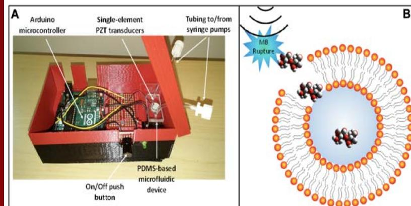
**Fig. 1.** A) Picture of the ultrasonic flow system. Ultrasound transducers are combined with PDMS-based fluidic devices inside a 3D-printed portable case to enable sequential and consistent loading of compounds across cellular membranes. B) Cartoon of microbubble (MB) rupture leading to active transport of compounds across cell membranes (not to scale)<sup>2</sup>.
