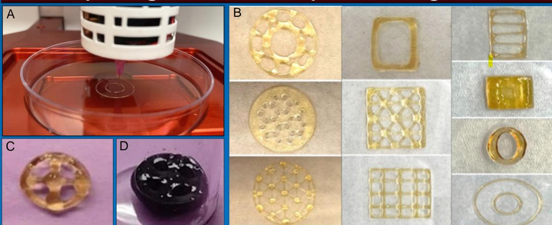
**Figure 2.** (A) 3D bioprinter<sup>2</sup> and (B) examples of 3D bioprinted shapes<sup>2</sup>. (C) 3D printed probiotic scaffold crosslinked with only CaCl<sub>2</sub>, compared with<sup>2</sup> (D) scaffold crosslinked with both CaCl<sub>2</sub> and genipin<sup>3</sup>.
