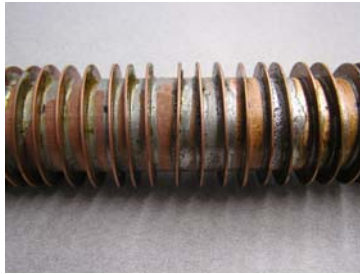
FIGURE 2.8 - Finned Condenser Section.
