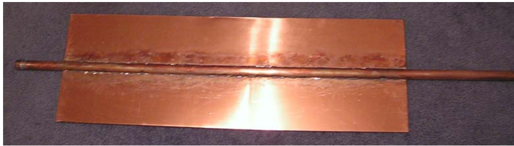
FIGURE 2.2 - Absorber Plate Construction.
