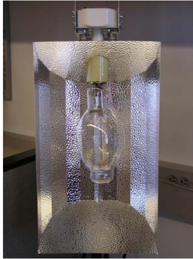
FIGURE 2.10 - Metal Halide 1000 Watt Solar Lights.
