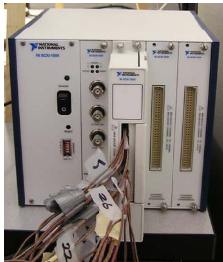
FIGURE 2.15 - SCXI Chassis With Digitizer And Module.
