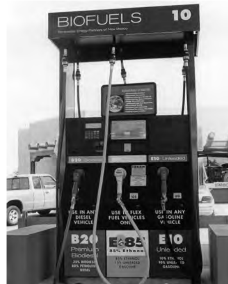
This fuel dispenser at a Santa Fe, New Mexico, station offers B20 biodiesel, E85 for flexible-fuel vehicles, and E10 for any vehicle that runs on gasoline (photo courtesy of Charles Bensinger and Renewable Energy Partners of New Mexico).
