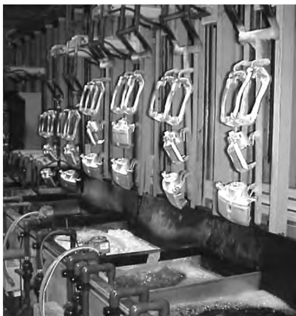
Technology diffusion at work in process water management with conductivity controllers installed on a manufacturer's plating line.
