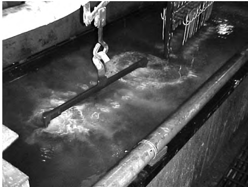
As illustrated in the photo, most metal processing companies use water intensive processes for surface preparation and plating.
