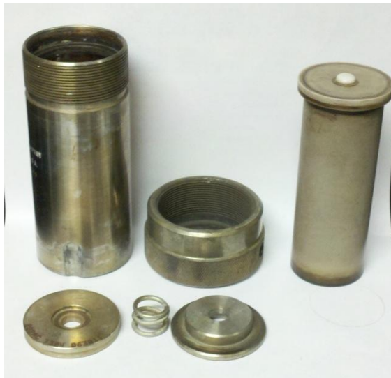
FIGURE 11 - Hydrothermal Autoclave with 50mL Teflon Vessel
