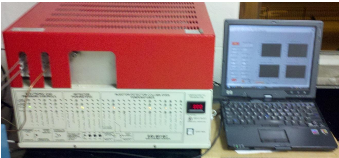
FIGURE 19 - GC-MS HP 5890 Gas Chromatograph equipped with 5970 Mass Selective Detector
