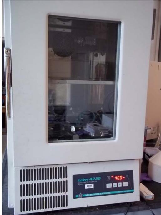
FIGURE 12: Innova 4230 Refrigerated Incubator Shaker
