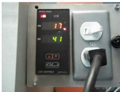
FIGURE 14: 8500 Series microprocessor based temperature control
