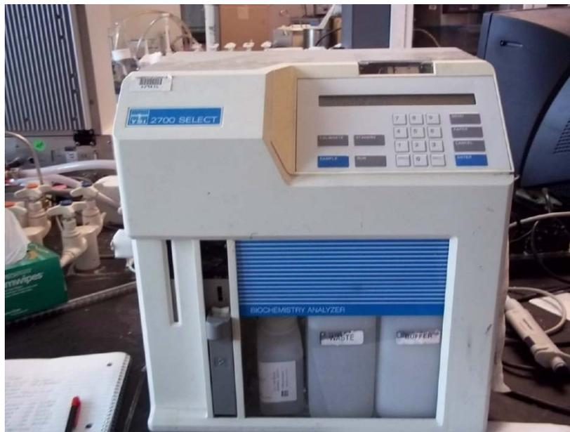
FIGURE 17: YSI 2700 Select Biochemistry Analyzer
