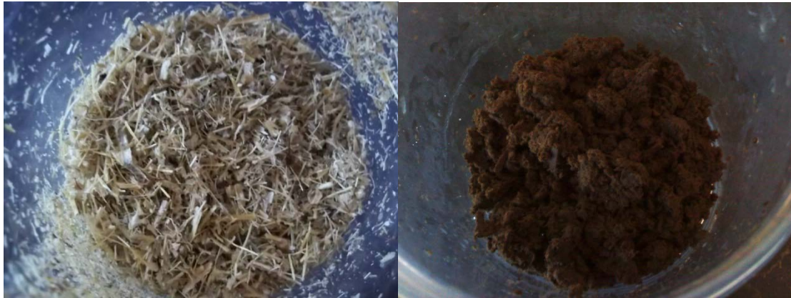
FIGURE 25: Dilute-base pretreated corn stover (left) compared to dilute-acid pretreated corn stover (right)
