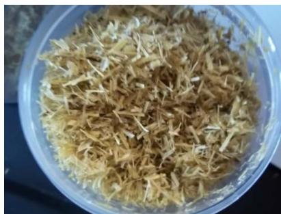
FIGURE 10: Dilute-base pretreated wheat after washing
