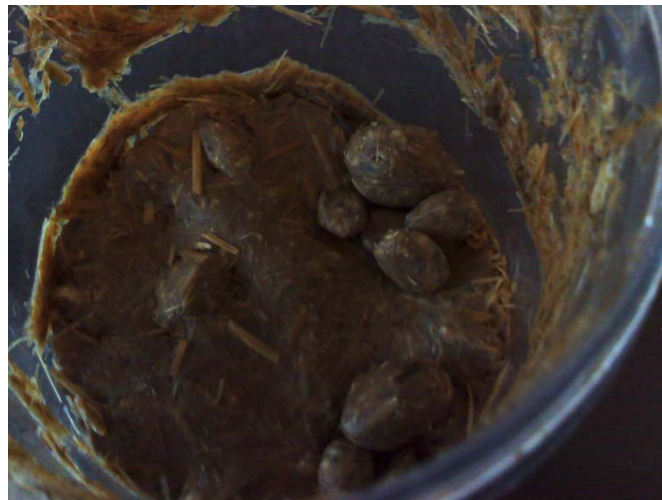
FIGURE 22: 30% solids corn stover from the mixer at 96 hours
