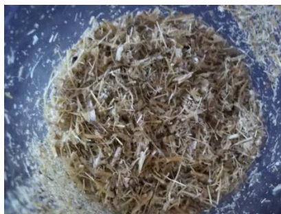
FIGURE 9: Dilute-base pretreated corn stover after washing
