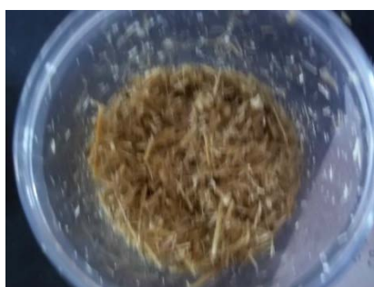
FIGURE 11: Dilute-base pretreated miscanthus after washing
