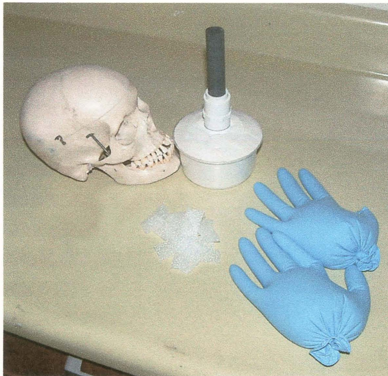
Figure 9. Materials used for imaging of skulls: gloves filled with water, skull holder and foam wedges, and skull.
