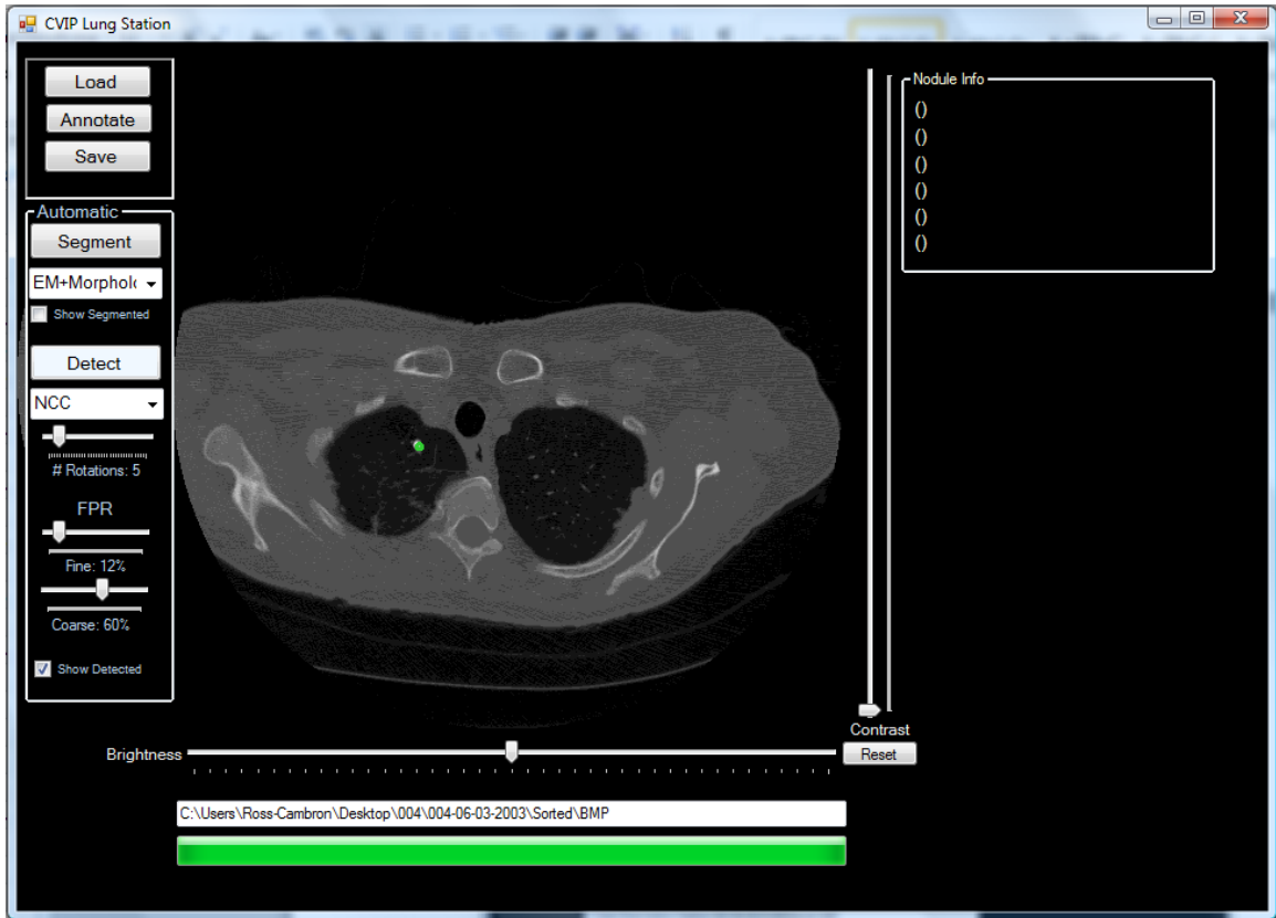
Figure 52: Updated detection results using the NCC with a Coarse FPR sensitivity of 0.6 and a Fine FPR sensitivity of 12%. The detection results yield a cluster of detected points surrounding a true, Calcified, Well-Circumscribed nodule. No false positives remain.
