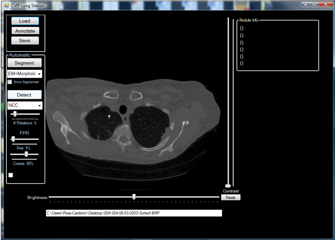
Figure 46: Viewing a raw CT slice in a scan that has previously undergone tissue segmentation. Notice the Show Segmented check box in the Automatic Toolbox. Enabling this check box isolates the lung tissue in the Slice View Panel.
