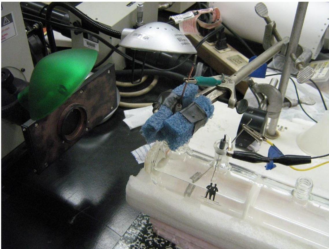
Figure 8. Photograph of a PEC cell with a three-electrode setup in front of a light source.
