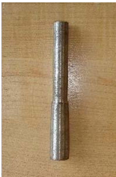
FIGURE 24. Steel rod used to secure modular body in lathe.
