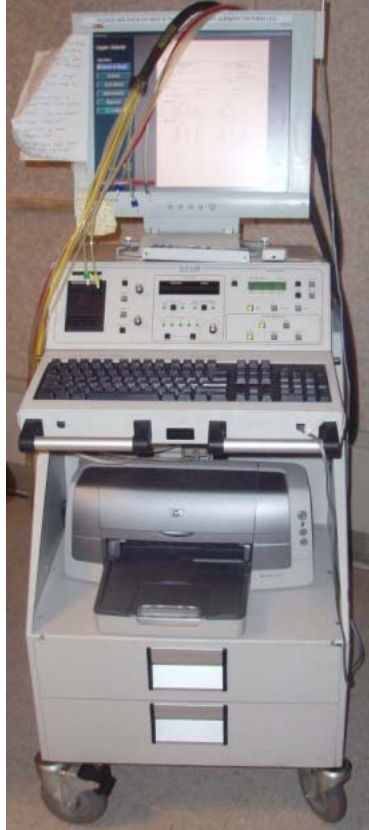
FIGURE 3 -- Flo-Lab 2100-SX for brachial index measurements
