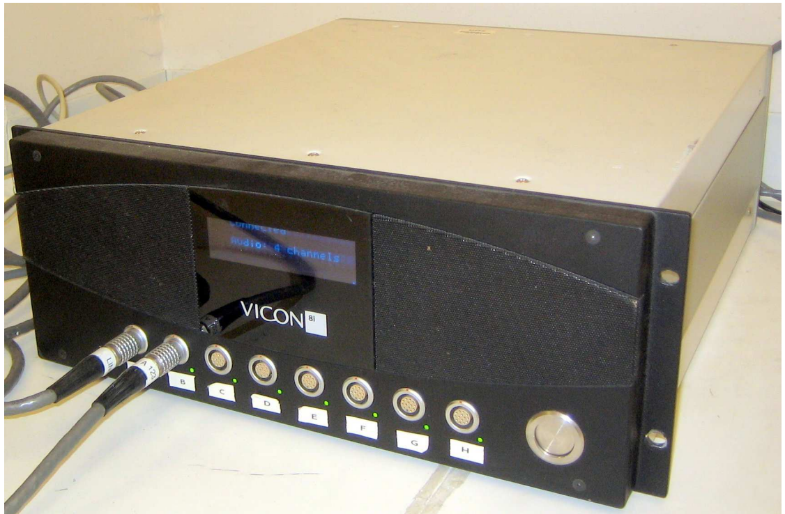
FIGURE 2.6: The Vicon V8 Datastation is the Frame Data Collection Unit
