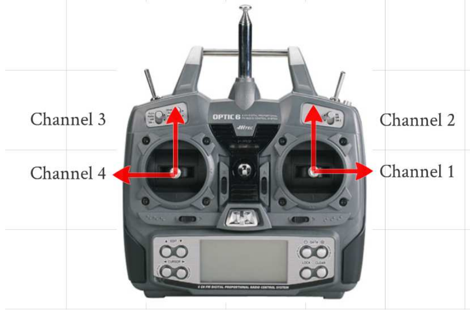
FIGURE 2.3: The RC transmitter channels. Channels 1 to 4 are roll, pitch, height, and yaw controls respectively. The fact that there are only four inputs to control a 6DOF vehicle makes the system under-actuated. Fortunately due to the symmetry of the quadrotor, the controls could be decoupled.
