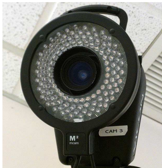
FIGURE 2.5: A Vicon M2 Camera with a maximum frame rate of 120 fps. The camera emits infrared to the field and receives reflections to locate and capture the objects.
