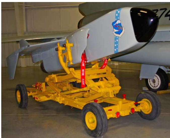
FIGURE 1.6: McDonnell ADM-20C-40-MC "Quail" could be carried by Boeing B-52 bombers and used as decoys.
