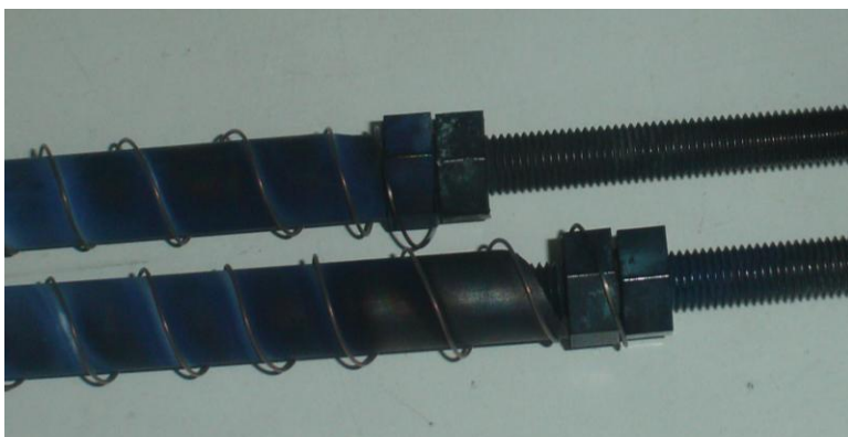
Figure 6: Detail of the electrical connection of the filament to the heating rods via molybdenum nuts.
