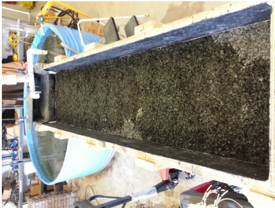
Figure 47: Experiment #11, 3% slope, 9 mm gap size, no aggregate between the pavers, after removing the pavers
