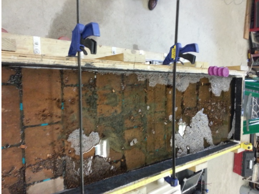
Figure 42: Clogged but not sealed, experiment #20, 5% slope, 6 mm gap size, #8 aggregate between the pavers
