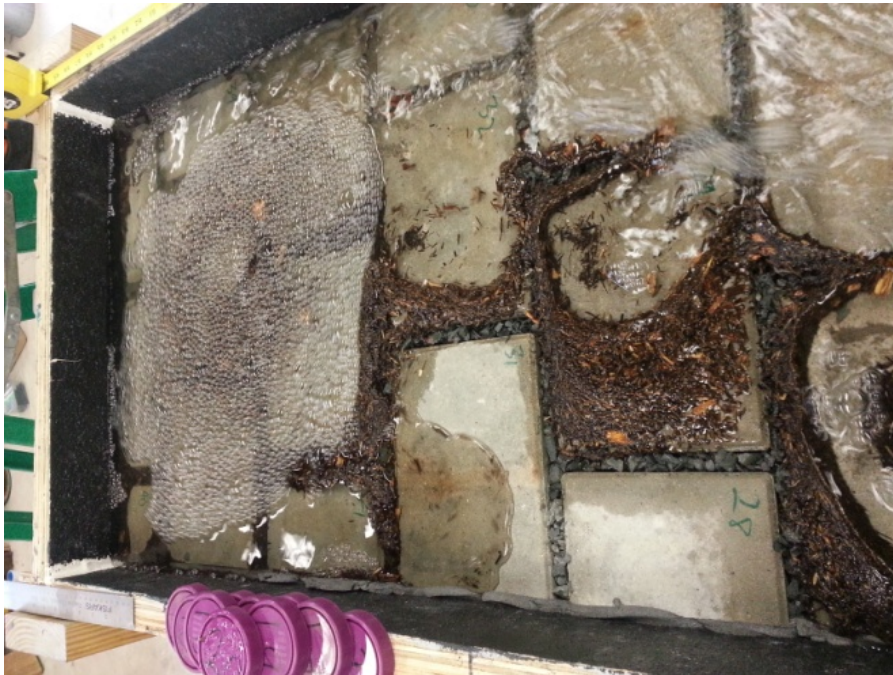
Figure 39: Clogged but not sealed, experiment #14, 3% slope, 6 mm gap size, #8 aggregate between the pavers
