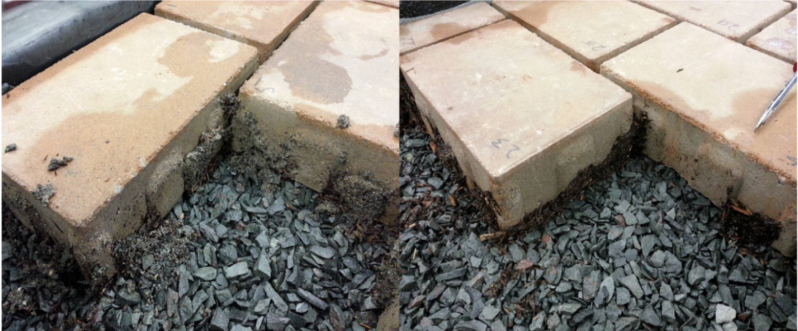
Figure 47: Experiment #11, 3% slope, 9 mm gap size, no aggregate between the pavers, after removing the pavers
