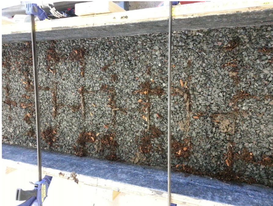
Figure 46: Experiment #19, 5% slope, 6 mm gap size, no aggregate between the pavers, after removing the pavers
