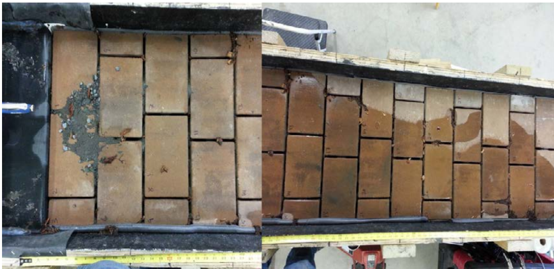
Figure 32: Experiment #1, 1% slope, 6 mm gap size, no aggregate between the pavers
