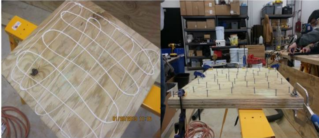
Figure 12: Construction of the flume's panels
