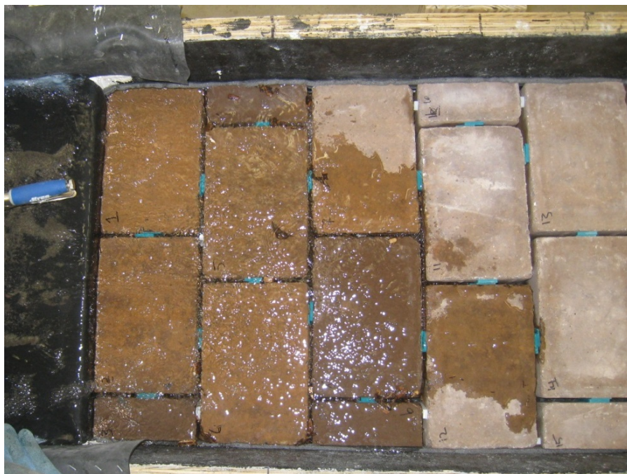
Figure 44: Experiment #1, 1% slope, 6 mm gap size, no aggregate between the pavers
