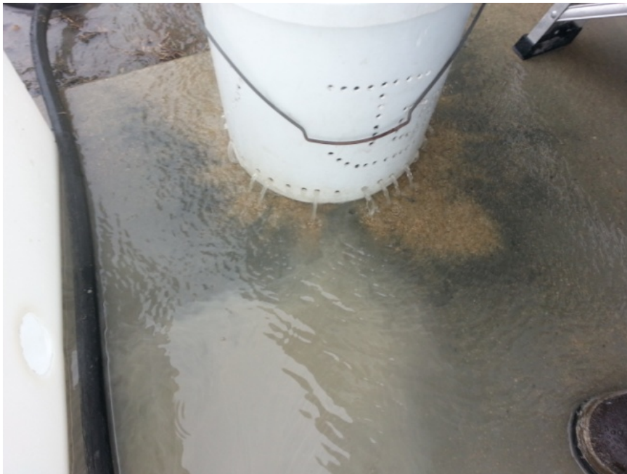
Figure 16: Washing the aggregate using a pressure washer
