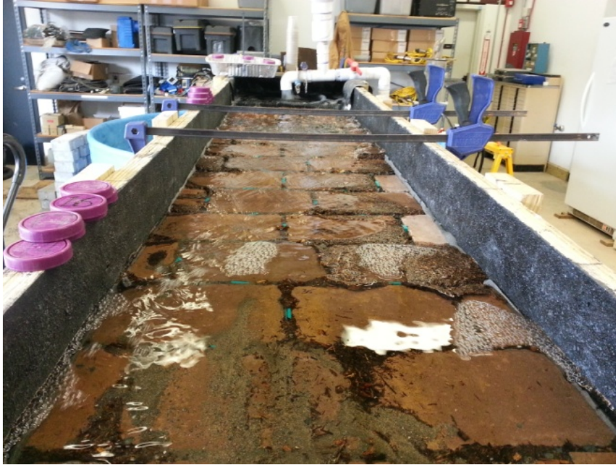
Figure 39: Clogged but not sealed, experiment #14, 3% slope, 6 mm gap size, #8 aggregate between the pavers
