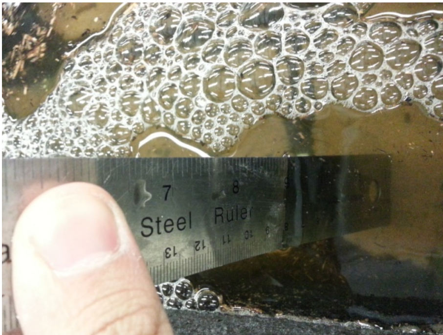
Figure 42: Clogged but not sealed, experiment #20, 5% slope, 6 mm gap size, #8 aggregate between the pavers
