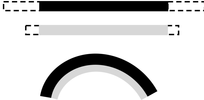
Figure 2.3: Linear bimetallic strip. The differing thermal expansion caused stress in the actuator when heated, and therefore deformation.
