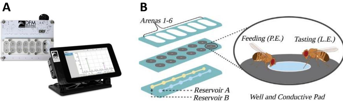
**Figure 2. Images of FLIC Apparatus.** (A) Photograph of FLIC Master Control Unit (MCU) and Drosophila Feeding Monitor (DFM) (Sable Systems, 2023) (B) Diagram showing the 12 arenas on the DFM, as well as the individual reservoirs associated with each row. Diagram also shows the difference between feeding events (proboscis extension) and tasting events (leg extension) (Philyaw et al., 2022).
