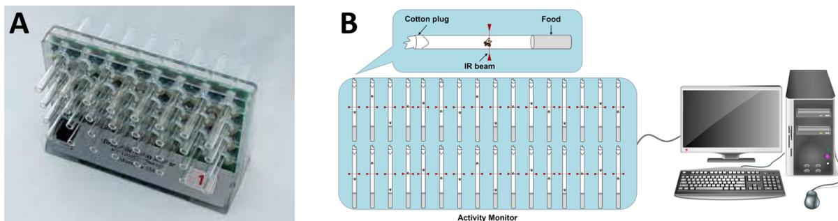
**Figure 3. Images of Assembled DAM System.** (A) Photograph of Assembled DAM board (Trikinetics, n.d.). (B) Diagram of DAM tubes with beam placement (Karam et al., 2022).
