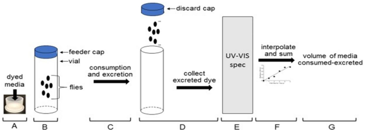
**Figure 1. Diagram of Modified Con-Ex Procedure.** Schematic of the steps for the Con-Ex method of *Drosophila* food quantification. Adapted from *Figure 1* (Shell et al., 2018).
