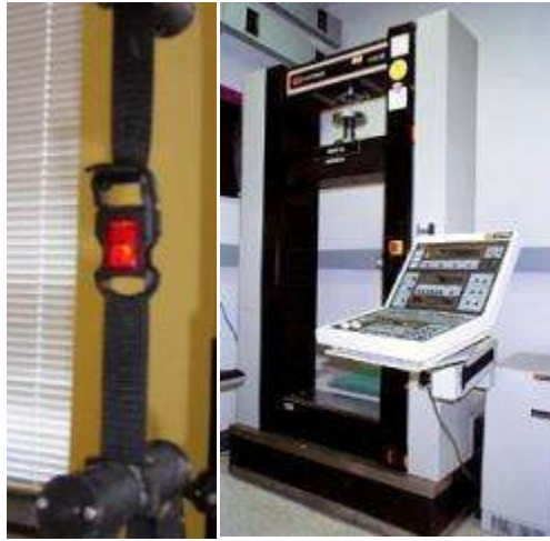
FIGURE 3 – Setup for Each Buckle Testing (Left) and the INSTRON 4500 (Right).
