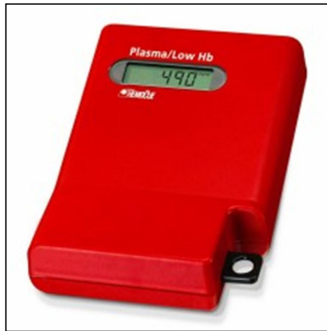
FIGURE 16 – HemoCue Plasma/Low Hb Photometer used in the trauma study to measure plasma free hemoglobin.
