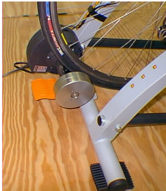
Figure 22. Bicycle rear wheel in contact with magnetic resistance unit.
