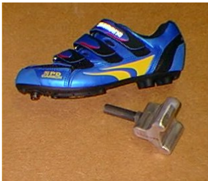
Figure 28. Three-point bending fixture and cycling shoe. Both sides of the fixture were designed as cylinders of radius 1 cm and length of 5.5 cm and placed lengthwise in the forefoot of the shoes.
