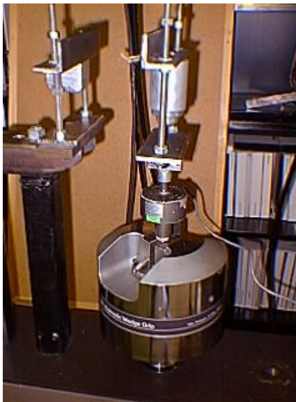
Figure 25. MTS machine in longitudinal bending arrangement. Seen below the fixture is a 200 lbf. (890 N) strain-gage force transducer.
