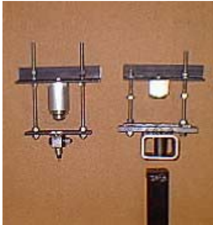
Figure 24. Longitudinal bending test fixtures. The fixtures were constructed per ASTM F-911 test standard.
