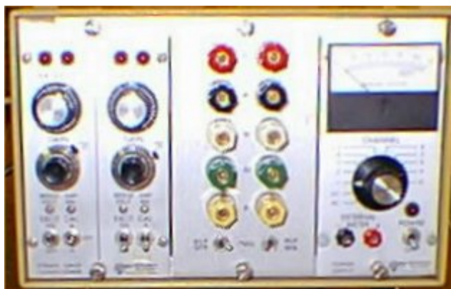
Figure 9. Wheatstone bridge circuit and amplifier.
