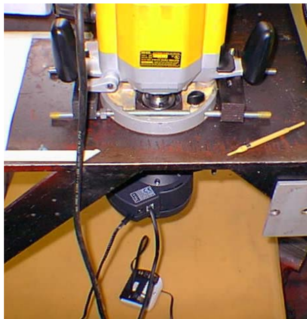
Figure 13. Router affixed to the steel table. The router was secured to the table, and the magnetic resistance unit was attached through the table to the router via a custom machined adapter.
