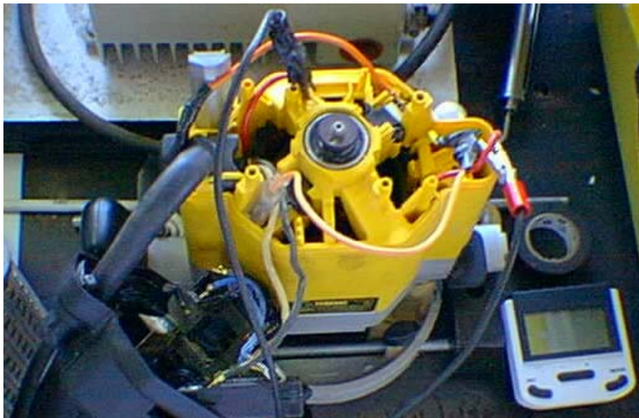
Figure 11. Rewiring of router motor for reverse rotation.
