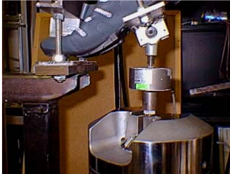
Figure 26. Longitudinal bending arrangement with shoe. Each shoe was flexed to a maximum angle of 20 degrees past the zero flex point.
