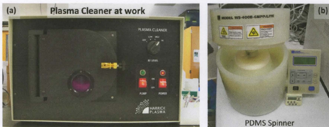
Figure 4.11. (a) Plasma ignited inside Harrick Plasma cleaner (b) PDMS spinner
