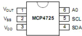
Figure 4.3: Pinout of the MCP4725 Analog Output IC.
