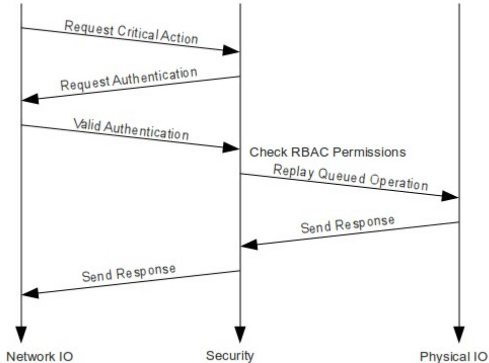
*Figure 3.3: IPC from Network Event to Physical IO, given proper role based access control credentials*
