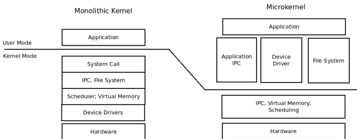
Figure 2.2: Monolithic and Micro- Kernel Architectural Differences.
