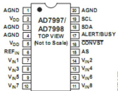
Figure 4.4: Pinout of the AD7997 Analog Input IC.
