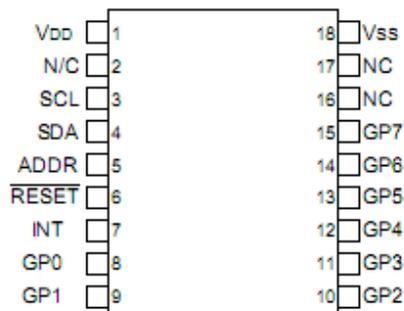
*Figure 4.2: Pinout of the MCP23009 Digital IO IC.*
