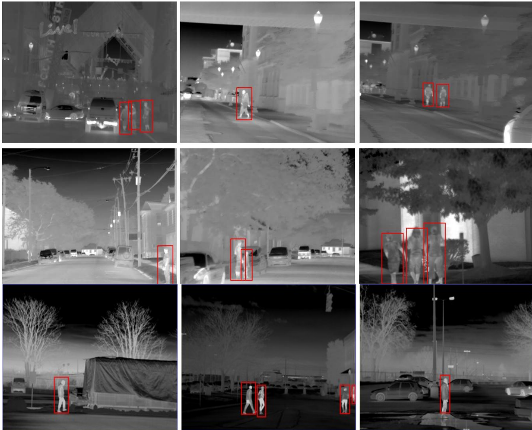
Figure 6.7. Some results for the obtained thermal imaging pedestrian detector at different weather conditions.
