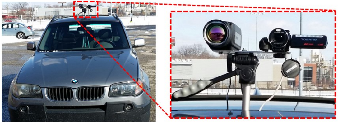
Figure 6.2. Setup used for data collection. A thermal camera and a visible camera are mounted on a vehicle as illustrated on the left part of the image. The right part of the image zooms on the cameras.
