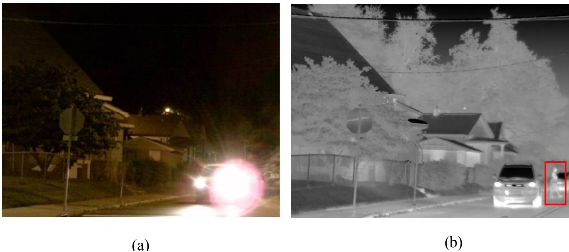
Figure 6.6. Night problems of visible image due to headlight glare. (a) A pedestrian is completely hidden by the glare in the visible image. (b) Corresponding thermal image with the pedestrian detected correctly using the obtained system.
