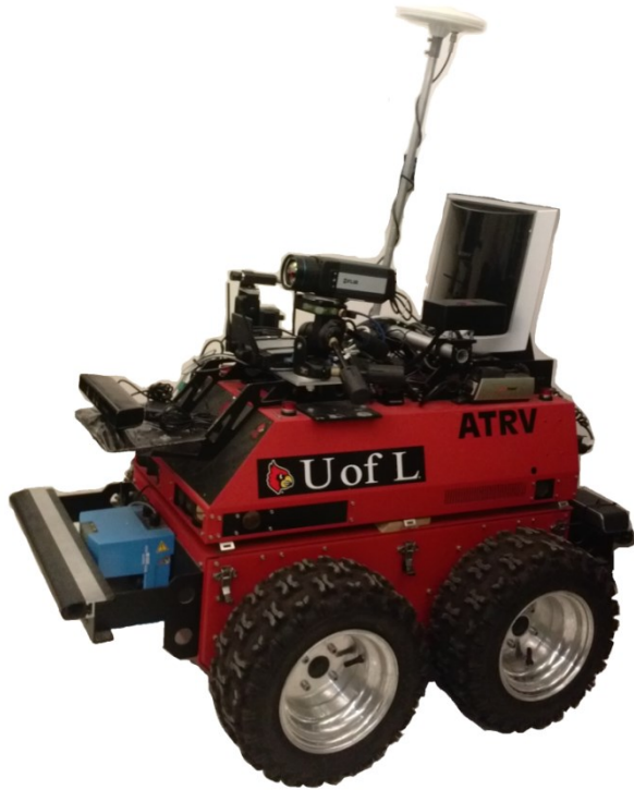
Figure 6.10. The ATRV2 with the FLIR LWIR thermal camera mounted on it.
