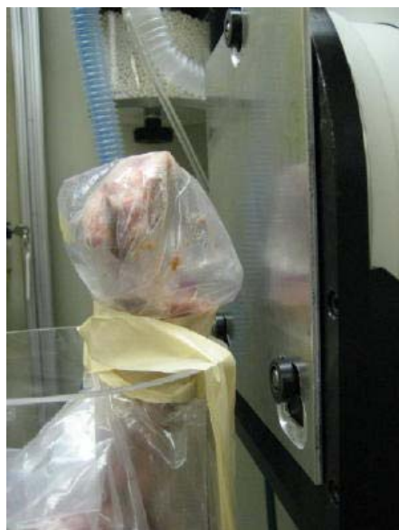
Figure 19. The proximal end of the pig femur specimen #2 set up with an aluminum sheet on the intensifier.
