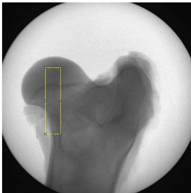
Figure 11. 2 nd region selected from digital X-ray images taken from the pig femur specimen #1.
