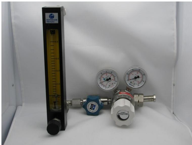
Figure 14 – Gas Regulator and Variable Area Flow Meter
