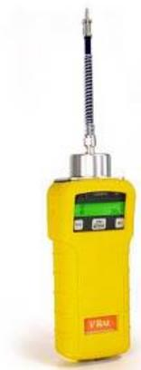
Figure 17 – PGM 7800 VRAE Multi Gas Monitor
