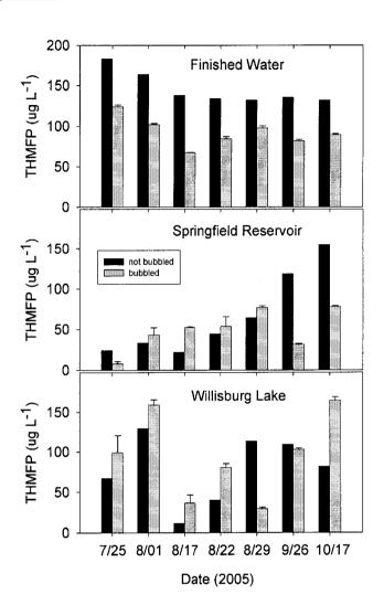
Results from the bench-top scale air oxidation experiment. Dark bars represent the THMFP of the samples that were split off and not bubbled while the lighter bars are the average THMFP of the three aerated samples. Finished water showed a significant (p < 0.0001) reduction in THMFP during each week sampled, while raw water from the hypolimnion of both lakes showed no consistent pattern of reduction by aeration, and often resulted in an increase in THMFP.
