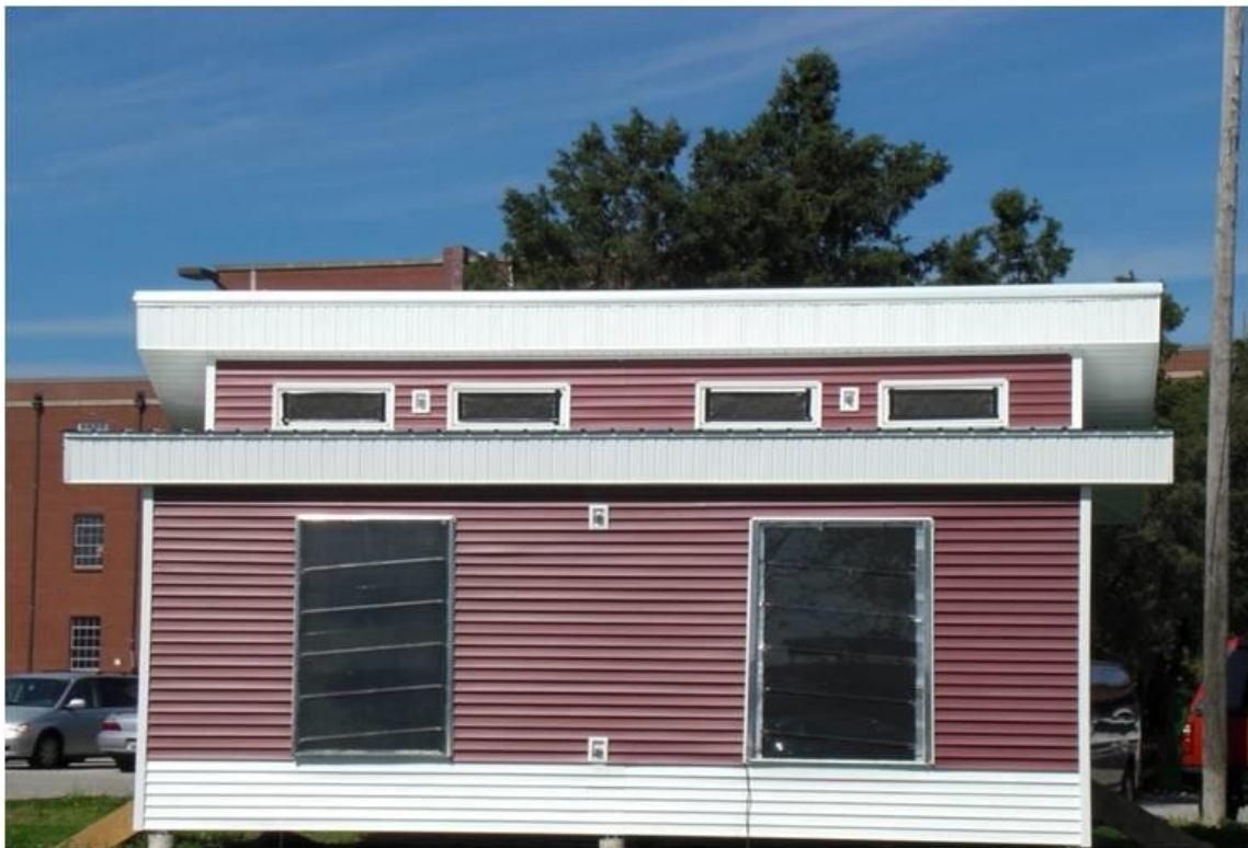
Figure 3.5. South view of the passive solar test facility. The collector for the previous prototype can be seen on the west (left) side of the wall, and the collector for the new prototype is on the east (right) side.
