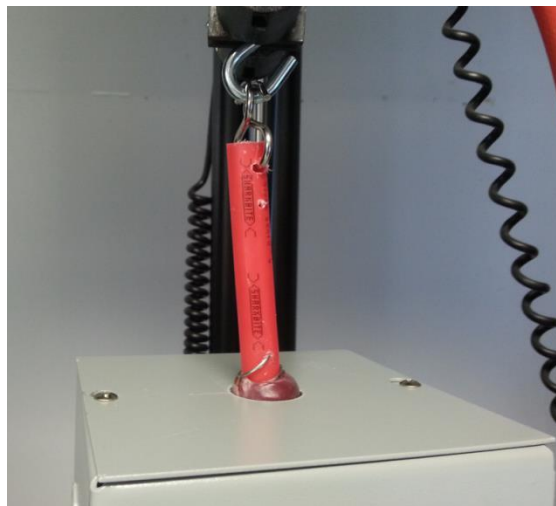
FIGURE 12- Tensile pull testing set up
