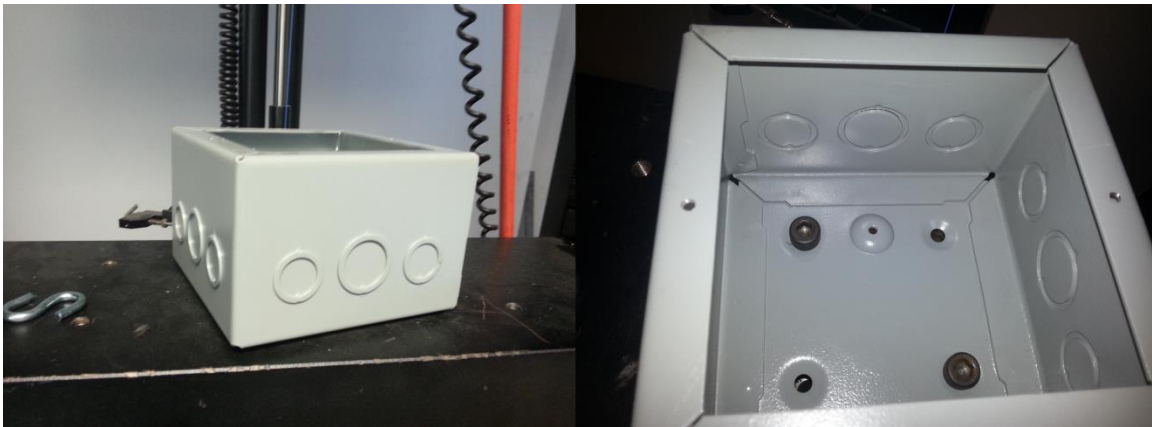
FIGURE 4- Electrical box on INSTRON base (left) and bolts securing box (right)
