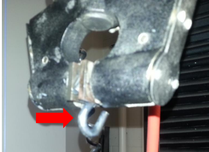
FIGURE 5- 1” S hook secured in upper grips of INSTRON
