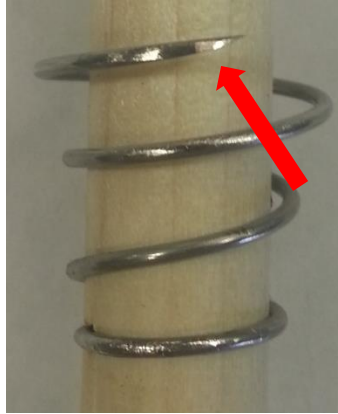
FIGURE 9- Sharpened spring and noticeable upwards angle
