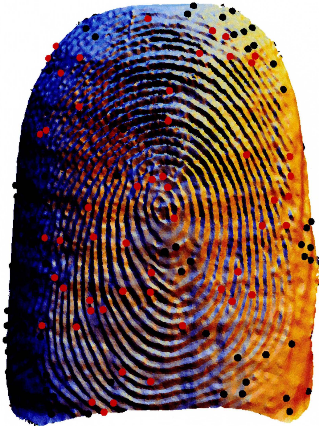
FIGURE 59 – Minutiae detection for the fingerprint in Figure 57. Black dots show minutiae associated with poor-quality areas and red dots show minutiae associated with high-quality areas.
