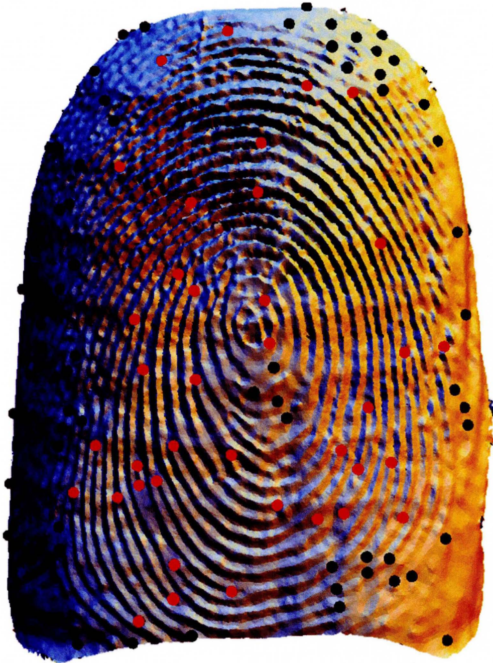
FIGURE 54 – Minutiae detection after applying quality map. Red dots show reliable minutiae detected in high quality areas and black dots demonstrate minutiae detected associated with poor-quality areas.
