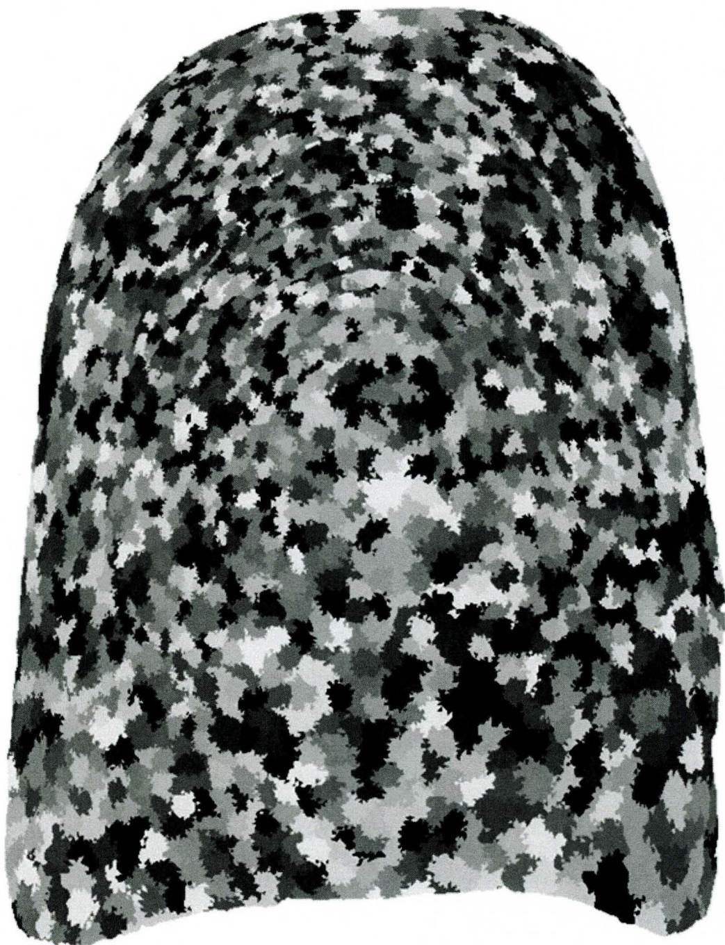
FIGURE 49 – Dividing the 3D fingerprint scan into blocks. Size of the blocks are 30 vertices. The blocks are shown by different color.
