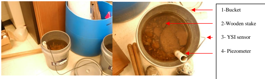
Illustration 7.4. Bucket with piezometer and wooden stake inside.
