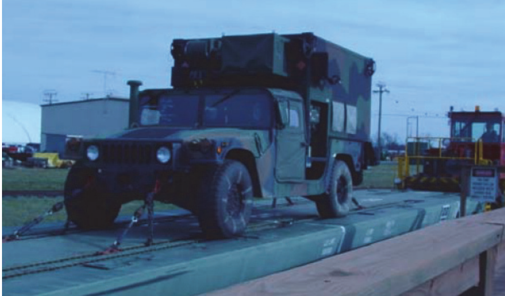
Figure 61. Rail impact test setup with HMMWV and rigid structure (ATC Rail Impact Facility, 2005 approx.)
