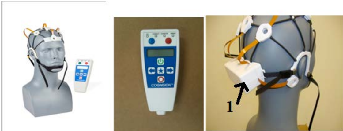
FIGURE 4 : The COGNISION™ 3000 Consists Of (A) Ten-Electrode Headset, (B) Control Unit, And (C) Data Acquisition. The Uberyoke (1. White Box) Contains Electronics For Signal Amplification, Analog-To-Digital (A/D) Conversion, And Control Logic (C).
