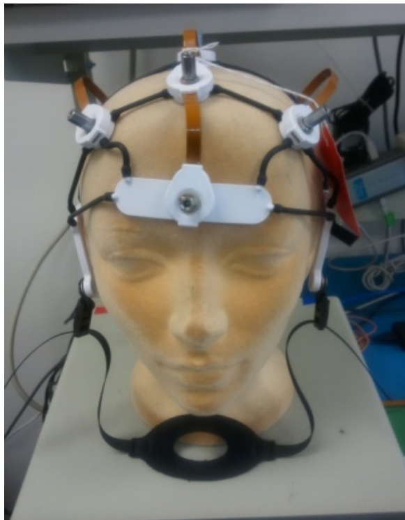
FIGURE 9 : Testhead, A Fixture Of The Testset Wearing The COGNISION Headset. This Fixture Is Used To Test The Headset Once It Is Assembled And Completed Systems. It Allows The Simulated Biosignal To Be Injected Into The Electrodes With Conductive Post That Articulate With The Electrode Pod's Monel Ring.
