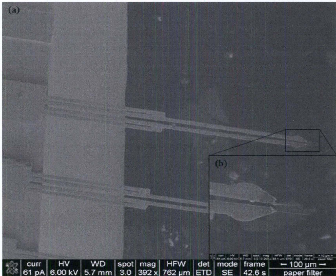
Figure 5.1 SEM images of the first design of nano-grippers: (a) full view; (b) close up view.
