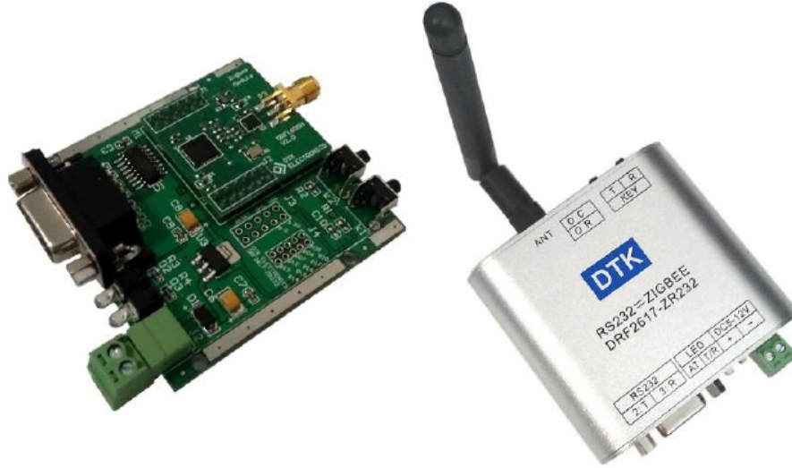
FIGURE 57: DTK RS-232 to ZigBee translational bridge [86].
