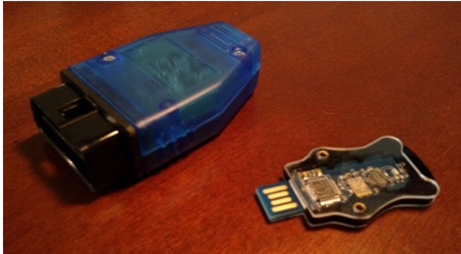
FIGURE 58: OBDII to ZigBee adapter for vehicle nodes.
