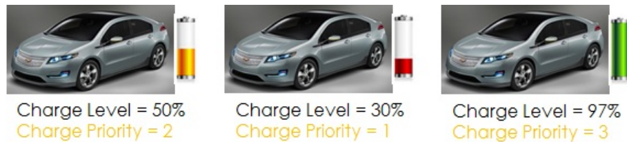
FIGURE 44: Prioritization of EV charging jobs based on vehicle state of charge.
