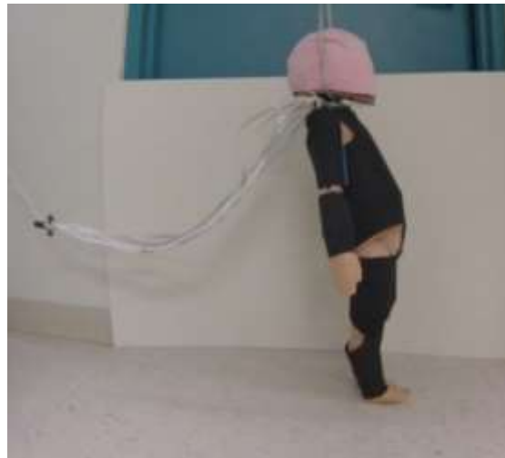
Figure 17: ATD in an upright initial position (scenario 1) for simulated rearward fall experiments
