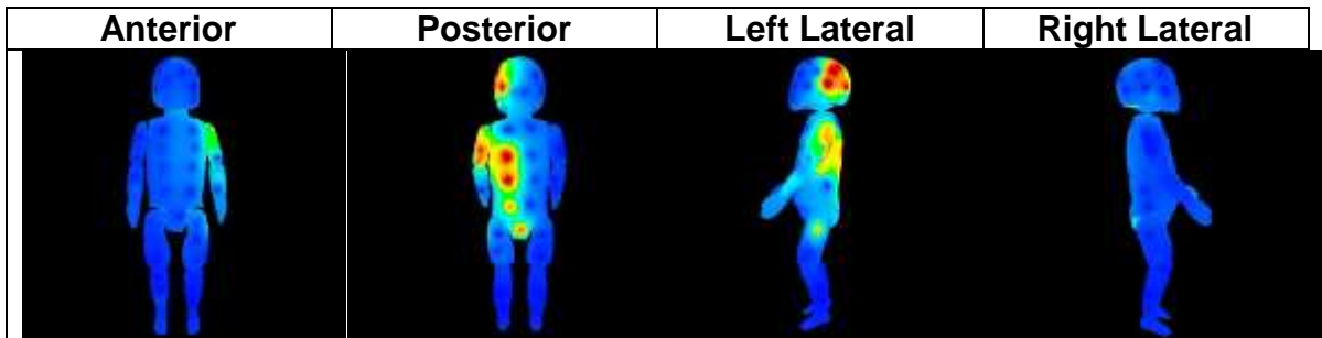
Figure 27: SBDS body map image corresponding to the FF36 bed fall impact where the colors and intensities vary depending on the level of force imparted to specific regions during the fall event
