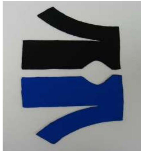
Figure 6: Neoprene patterns (top and bottom layers) cut for the prototype matrix sensor that would wrap around the forearm.
