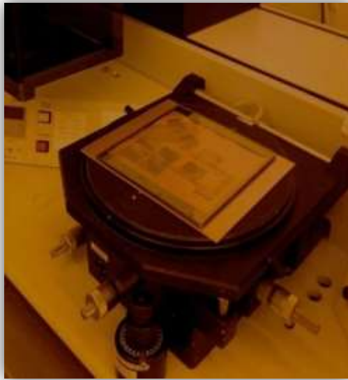
Figure C4: Glass photomask aligned over the photoresist coated copper substrate prepared for UV exposure.
