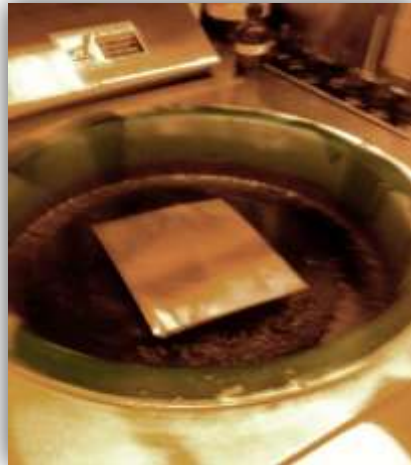
Figure C2: Copper substrate positioned within rotating machine tub after application of the photoresist.
