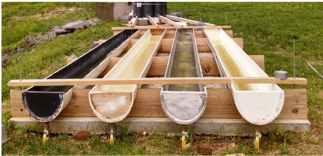
Figure 3.6 SODIS Troughs Setup and Out Flow Control
