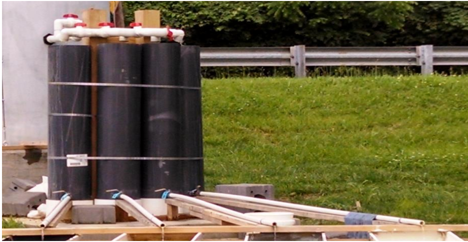
Figure 3.3 Filter Arrangement Showing Inflow and Outflow Controls
