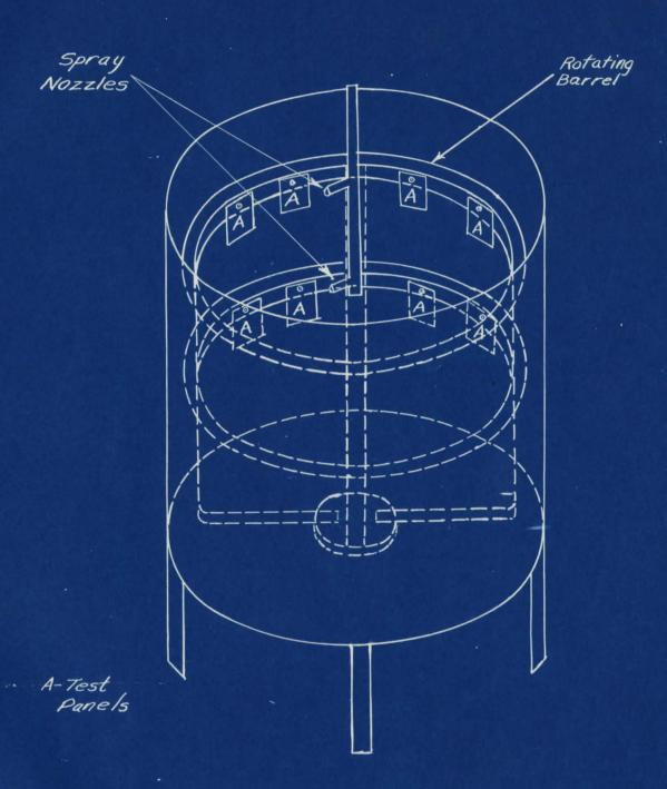
FIGURE 1 ACCELERATED WEATHERING UNIT
