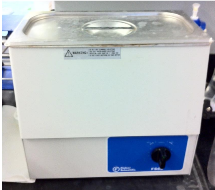
FIGURE 1—Ultrasonic Cleaner used to indirectly mix solutions
