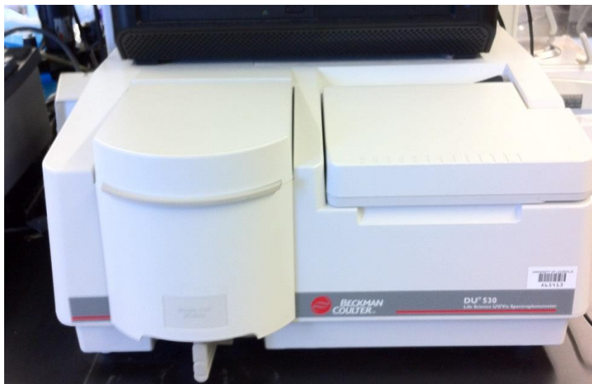
FIGURE 3—Spectrophotometer used for absorbance measurements.
