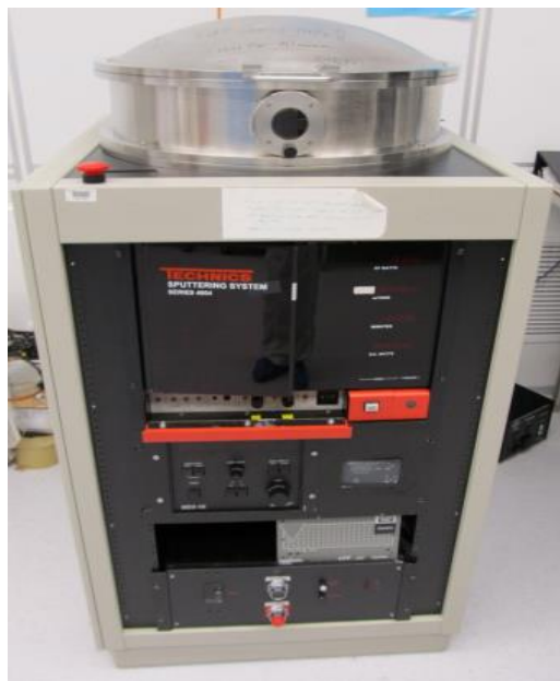
Figure 3.1. Technics 4604 Sputter Coating System used for silicon film deposition
