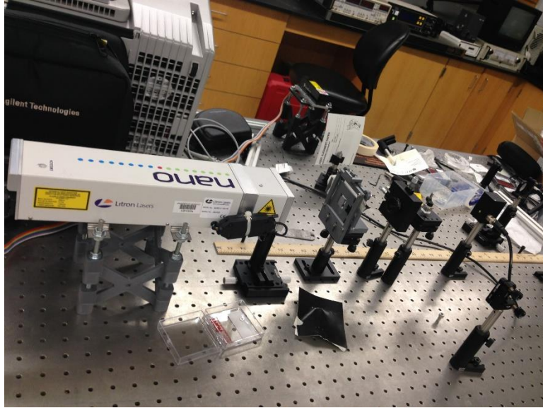
Figure 2.6. Experimental set-up of laser spallation system
