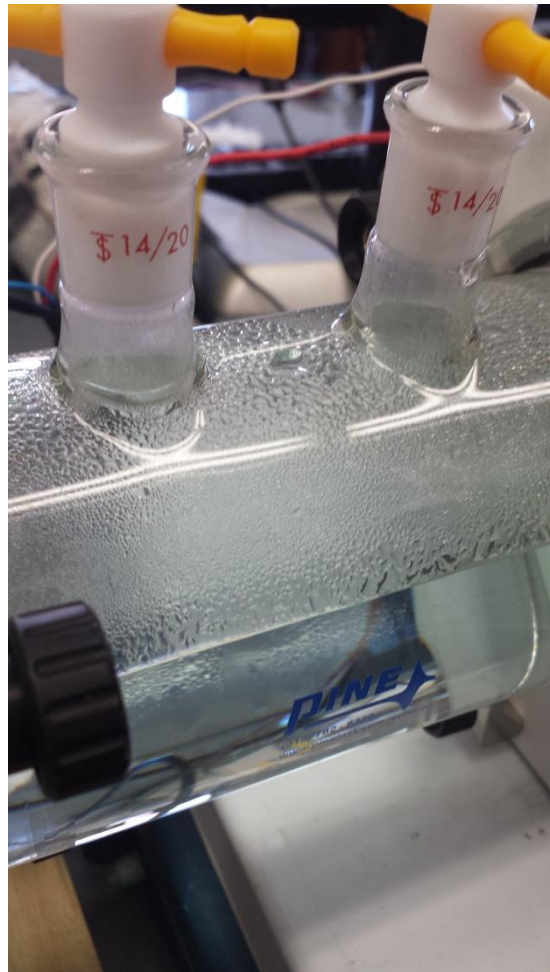
Figure 36. Condensation of electrolyte during testing of 0.01M \text{CuSO}_4 \cdot 5\text{H}_2\text{O} based thermocell.
