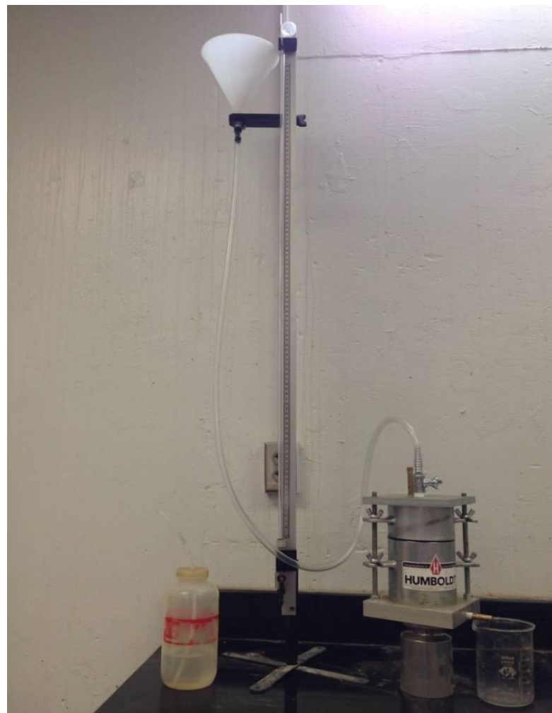
Figure2.11 The constant head testing system
