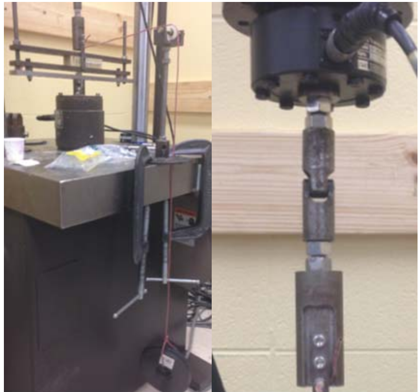
Figure 2: Wide view of the testing setup with counterweight and large C-clamps (left) and MTS Strain Gage / universal joint interface at the top of the setup (right).
