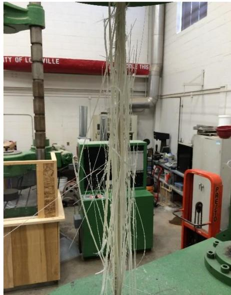
FIGURE 17 – Failure of GFRP Tension Specimen
