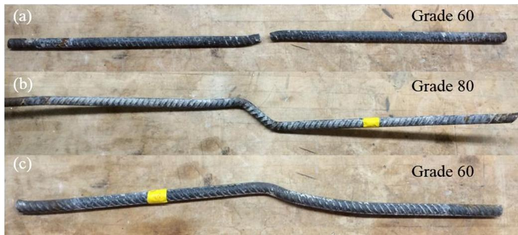
FIGURE 22 – Steel Failure and Deformation: (a) 135°; (b) 45°; (c) 90°
