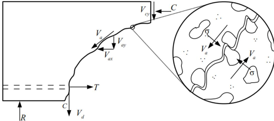
FIGURE 5 – Detail of Aggregate Interlock (Wight and MacGregor 2012)
