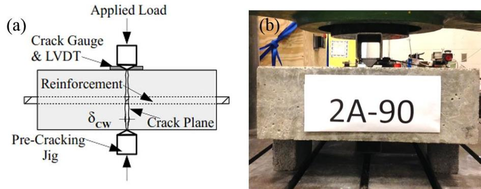
FIGURE 14 – Pre-Cracking Test: (a) Detail; (b) Test Specimen
