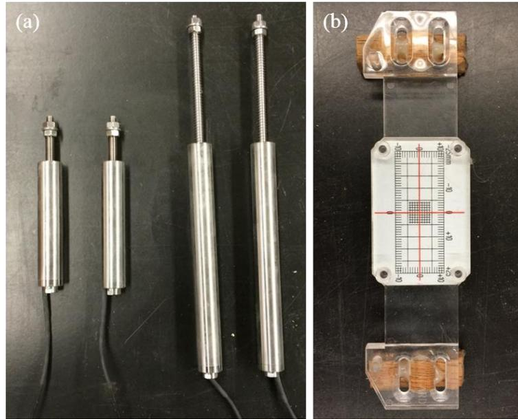
FIGURE 13 – Instrumentation: (a) LVDTs; (b) Standard Crack Gauge
