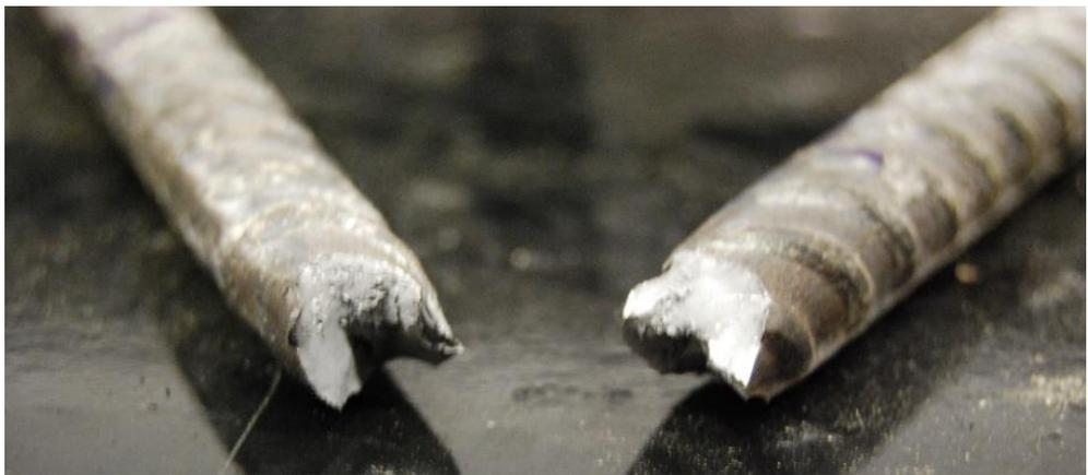
FIGURE 19 – Failure of Steel Tension Specimen
