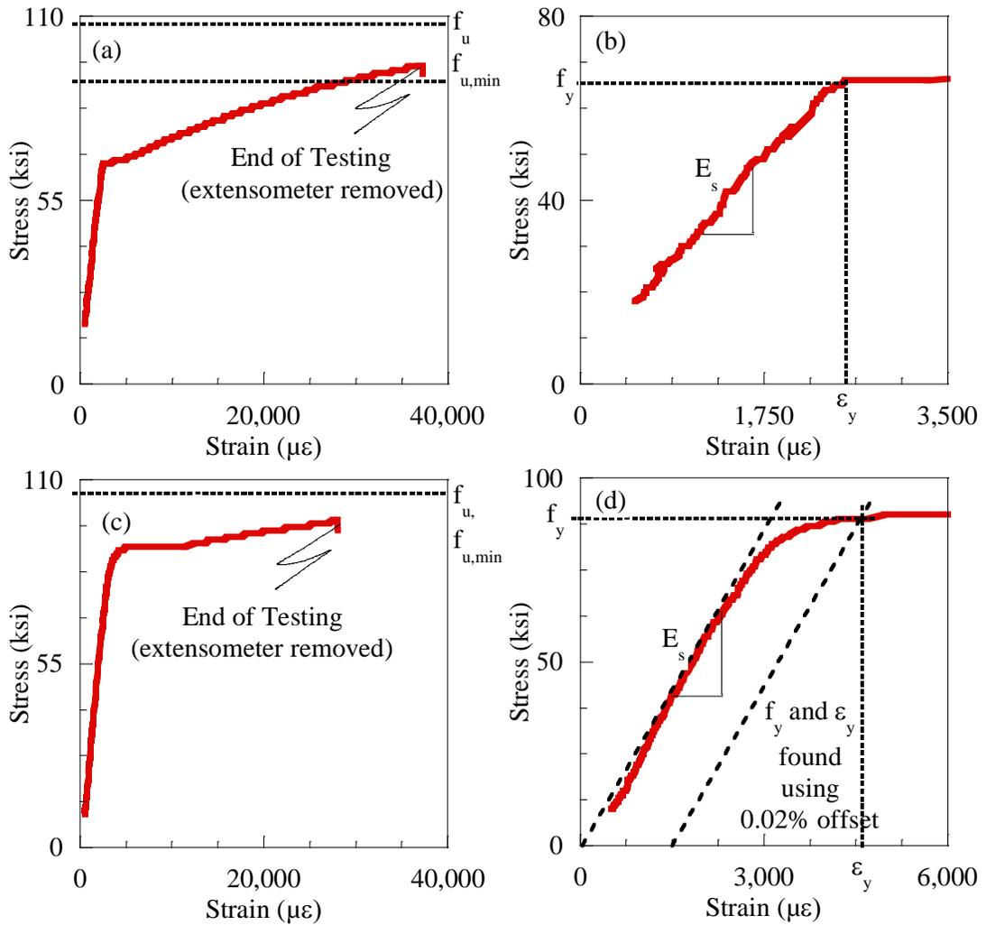
FIGURE 20 – Steel Stress-Strain Curves: (a)  $f_u$  and  $f_{u,min}$  (Grade 60); (b)  $E_s$ ,  $f_y$ , and  $\epsilon_y$  (Grade 60); (c)  $f_u$  and  $f_{u,min}$  (Grade 80); (d)  $E_s$ ,  $f_y$ , and  $\epsilon_y$  (Grade 80)
