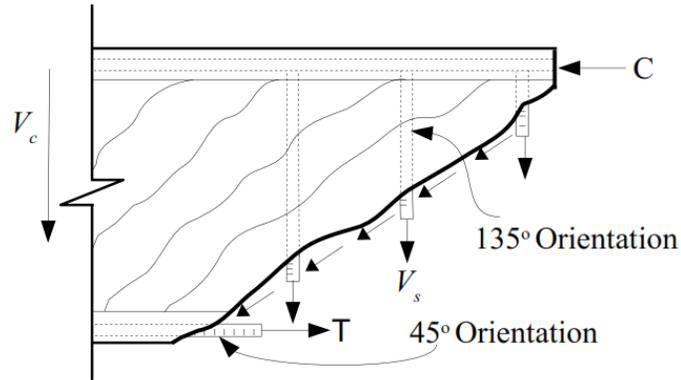
FIGURE 7 – Representative Reinforcement Angles in R.C. Beam
