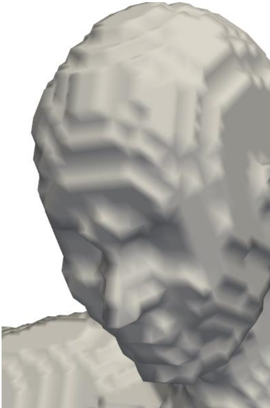
FIGURE 14 - Surface obtained by marching cubes algorithm. Note the jagged transitions.
