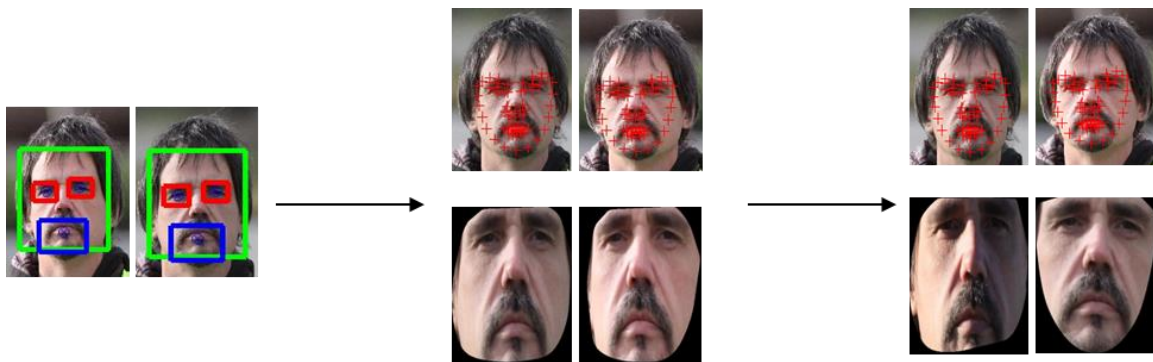
FIGURE 31 - The output in each step in face cropping for a good candidate in initial and final face cropping
