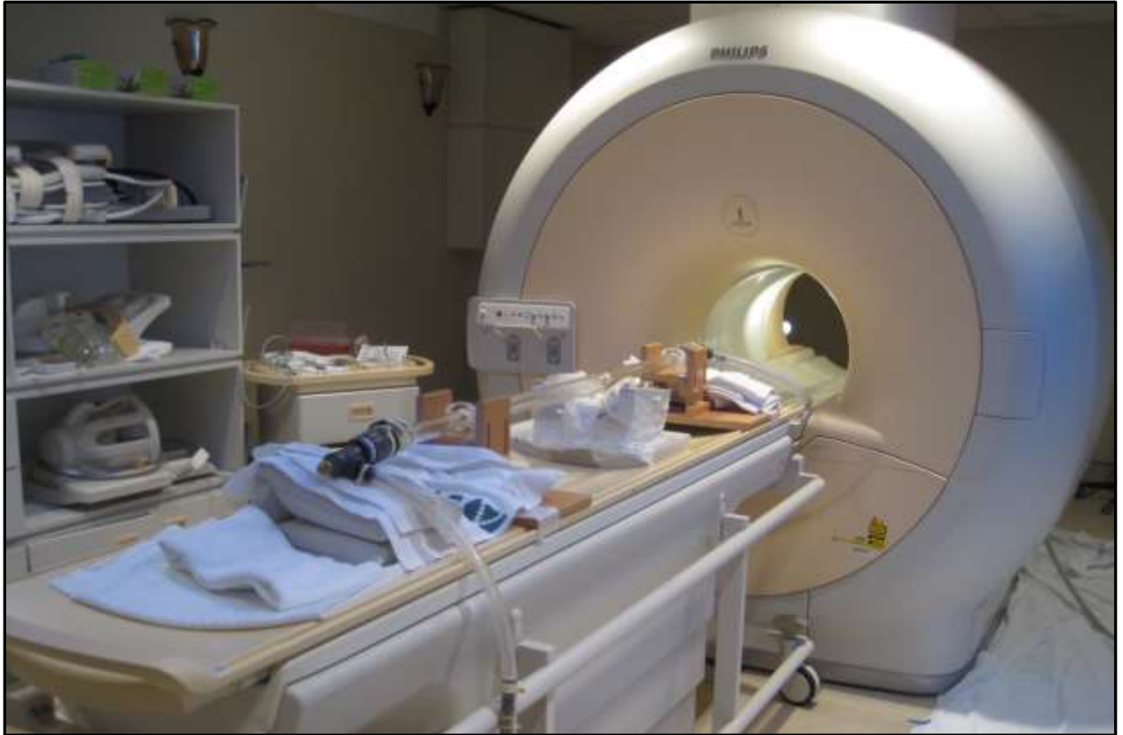
Figure 55 Actual set up of flow phantom inside MRI scanner. The pump and control unit are in the lower right hand corner of the room and cannot be seen in the picture.
