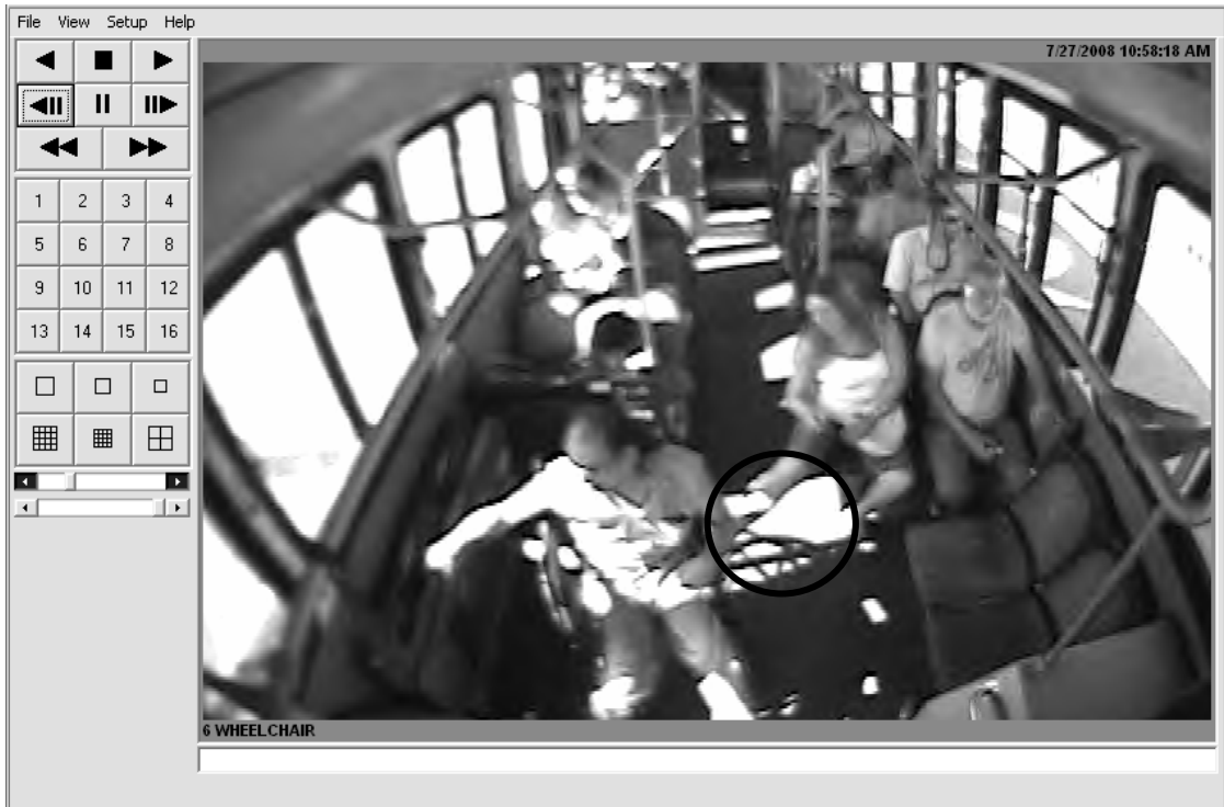
Figure 6. Case 2: Manual wheelchair passenger and wheelchair rotated into aisle as LATV performed a right turn. Wheelchair passenger stabilized himself by placing both feet on the floor and using his right arm to grab the folding-seat while an ambulatory passenger used her foot to prevent additional lateral excursion of the wheelchair. (View from LATV front).
