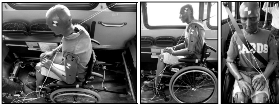
Figure 2A. Typical test setup of 50 th percentile ATD seated in manual wheelchair with four tie-downs and lap and shoulder belt applied. Low-g accelerometers were mounted in the ATD head, chest, and pelvis as well as on the LATV floor (at securement station). Load cells were used to measure webbing tension in the tie-downs and lap and shoulder belts.
