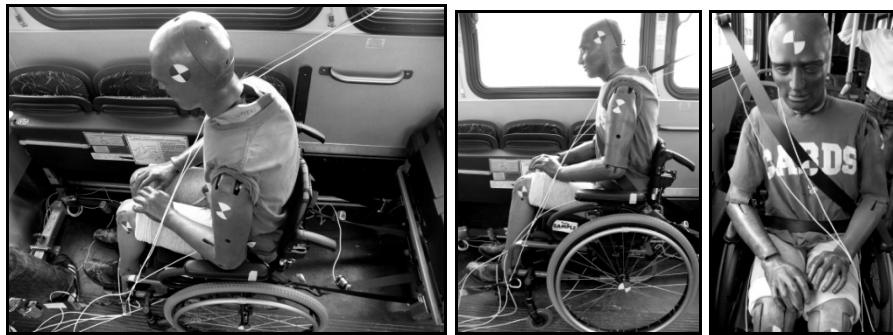
Figure 1. Test setup of 50 th percentile ATD seated in manual wheelchair with four tiedowns and lap and shoulder belt applied. Low-g accelerometers were mounted in the ATD head and chest, the wheelchair CG, as well as on the LATV floor (at securement station). Load cells were used to measure webbing tension in the tiedowns and lap and shoulder belts.
