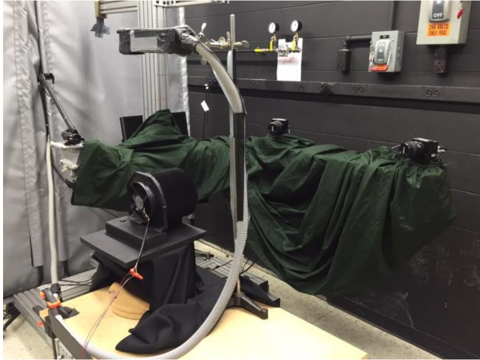
Figure 4.8: PIV setup for roll MCHX (Add arrows and labels)
