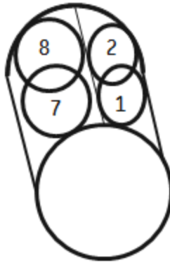
Figure 5.14: Vane anemometer measurement location schematic for roll MCHX
