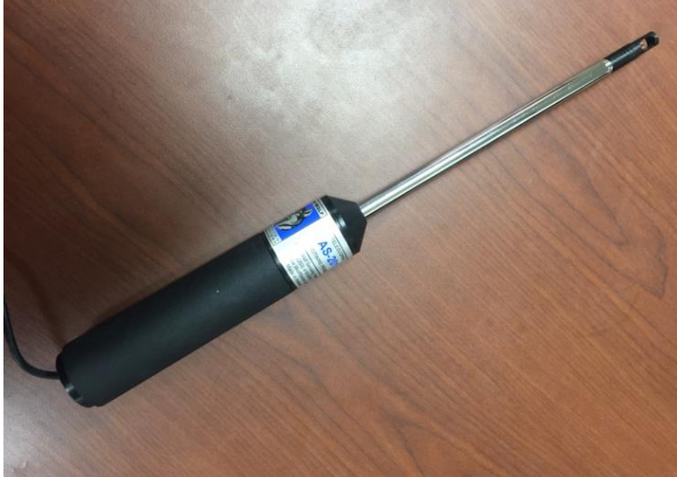
Figure 4.12: Graywolf AS-201 hotwire anemometer used to measure local airflow rates
