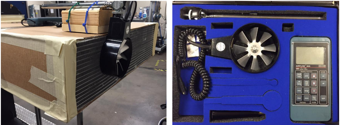
Figure 4.7: Airflow AV6™ digital handheld vane anemometer (R) shown measuring local velocity on a flat MCHX (L)
