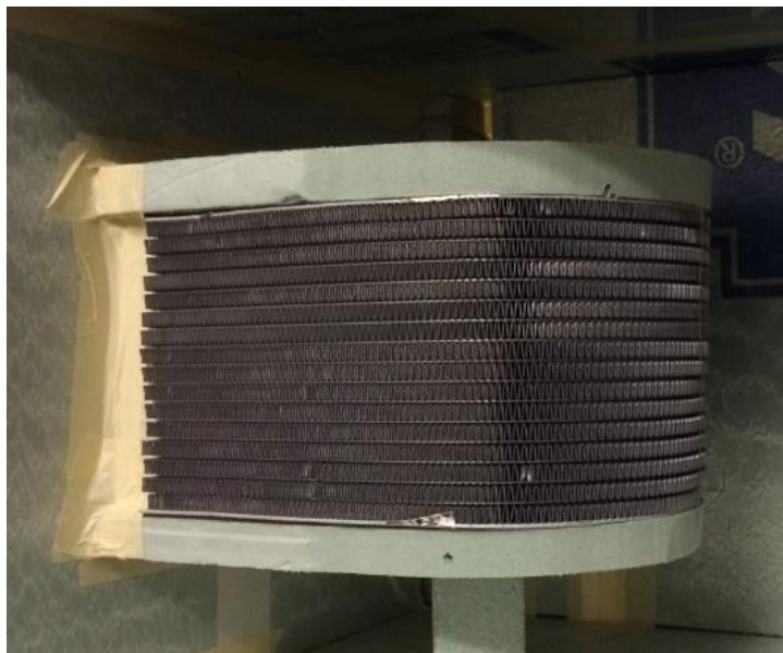
Figure 5.2: U-shaped MCHX installed in water calorimeter
