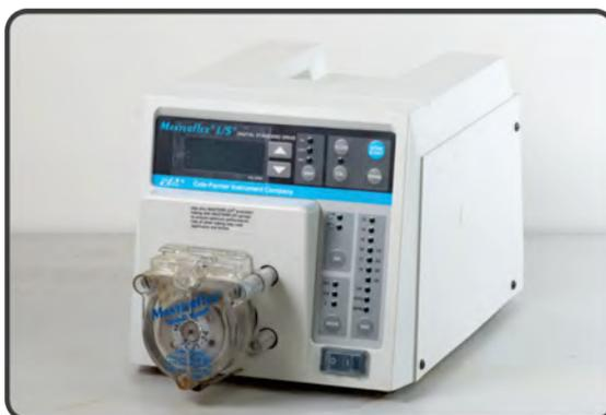
FIGURE 21 - Masterflex L/S digital peristaltic pump used to circulate the electrolyte.
